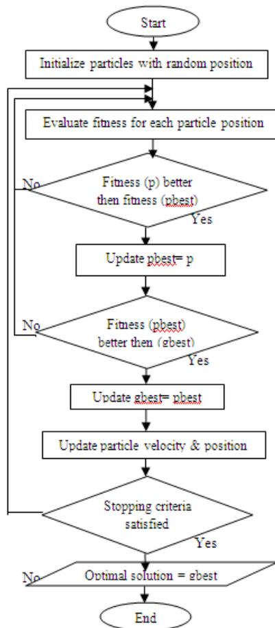
Fig. 3 Particle Swarm Optimization Algorithm flowchart
