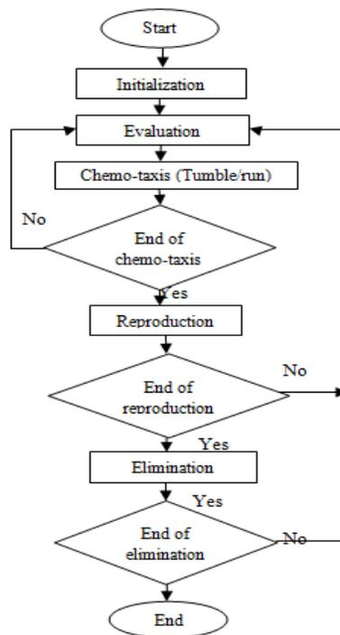
**Fig. 4 Bacterial Foraging Optimization algorithm flowchart**
