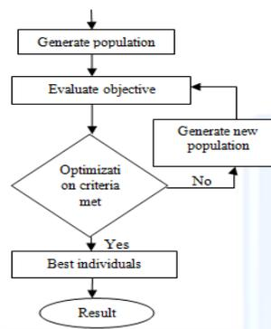
**Fig. 1 Structure of Evolutionary Algorithm**
