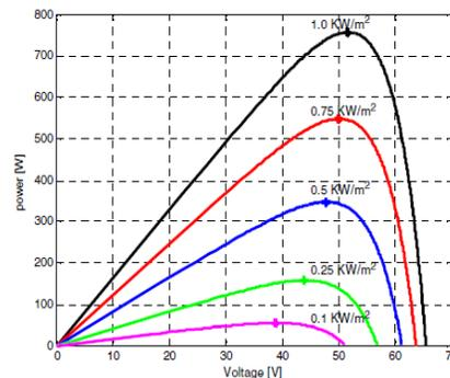
**Fig. 8: P-V Characteristics of PV Module**
