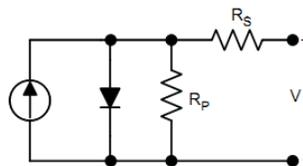
**Fig.2 single diode PV model**
