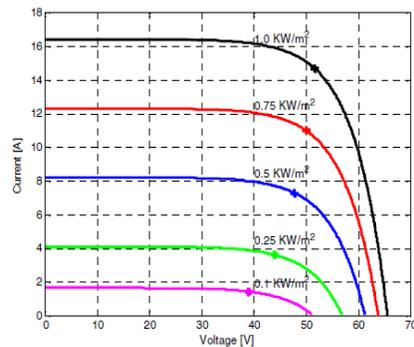
**Fig. 7 I-V Characteristics of PV Module**
