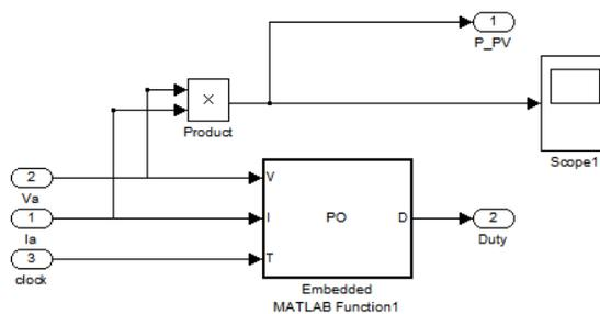
**Fig. 6 Block diagram of modeled MPPT system**
