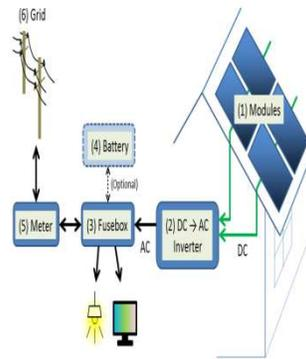
**Fig.1 Basic photovoltaic system**
