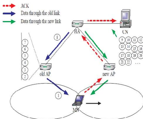
Figure 3: Packet Burst Caused by Handovers
