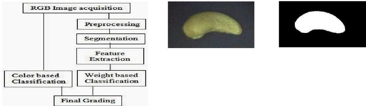
Fig. 1. (a) System Architecture (b) RGB top view (c) RGB front view (d) Binary top view (e) Binary front view of cashew kernel
