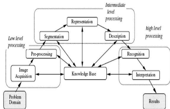
Fig. 2. Different levels in the image processing process (Sun, 2000).
