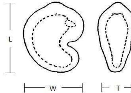
Figure 1: Length(L), Width(W) and Thickness (T) of the cashew kernel.
