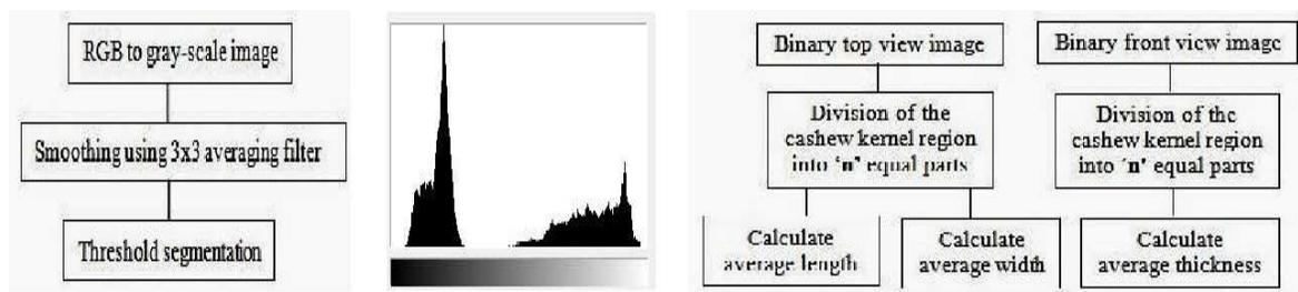
Fig. 2. (a) Preprocessing and Segmentation (b) Bi-modal Histogram of cashew kernel image (c) Morphological feature extraction
