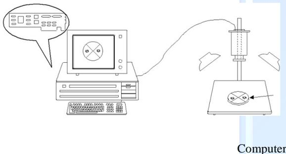
Fig. 1. Components of a computer vision system (Wang & Sun, 2002a).
