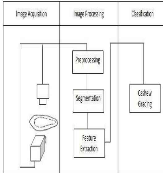
**Figure 2: Schematic representation of cashew grading system**
