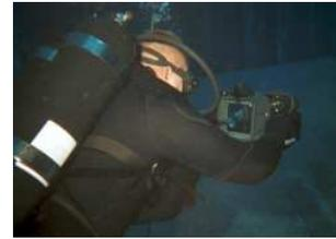
for use by a diver. Integrated Navigation Sonar System (INSS) is a small flashlight-shaped handheld sonar for divers that displays range.
