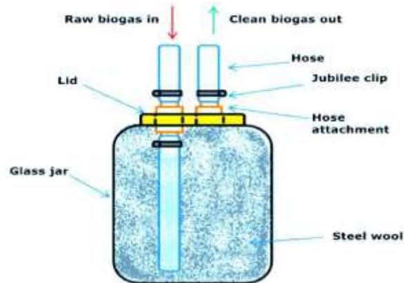
*Fig 3: Hydrogen Sulphide Remover*
