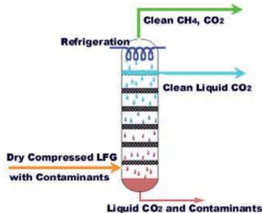
Fig 2: Schematic view of the CO<sub>2</sub> Wash
