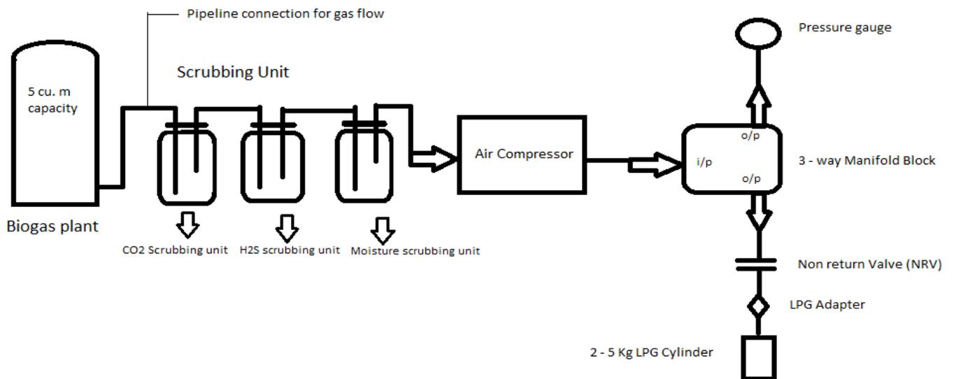
**Fig 1: Typical arrangement of biogas enrichment plant.**
