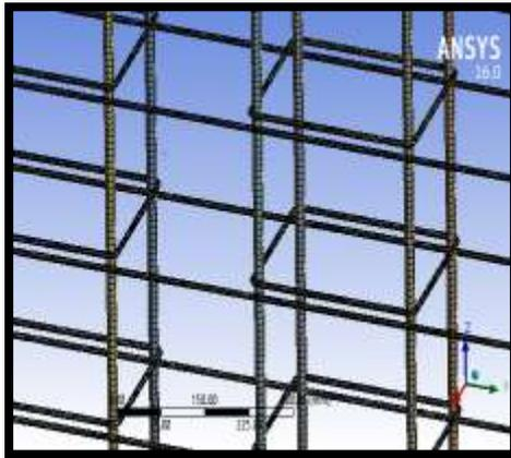
Figure 4 . Meshing of reinforcement 6mm
