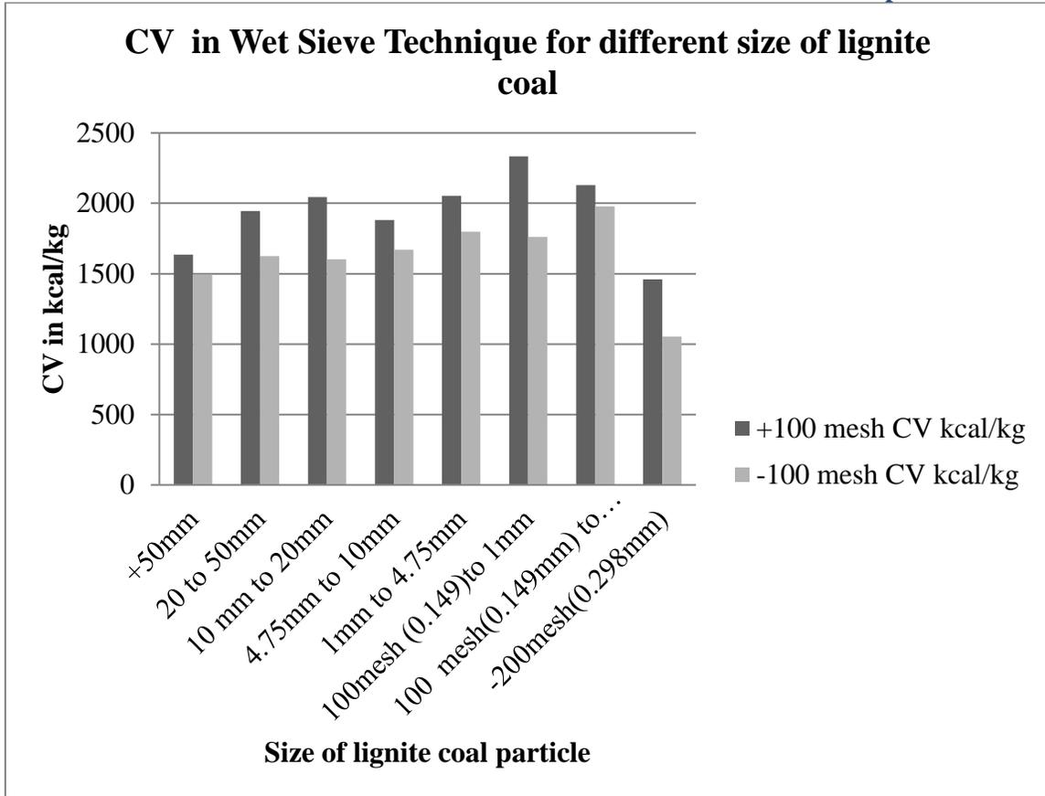
Fig. 4 The representation of CV kcal/kg in wet sieve Technique for +100 mesh size and -100 mesh fine size 0.298 mm to 50 mm
