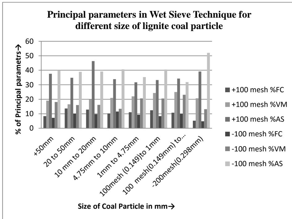
Fig. 2 The representation of principal parameters in wet sieve technique for +100 mesh and -100 mesh fine size.
