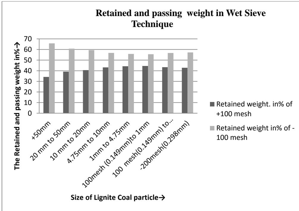
Fig. 1 The representation of retained and passing weight in wet sieve technique for +100 mesh and -100 mesh size
