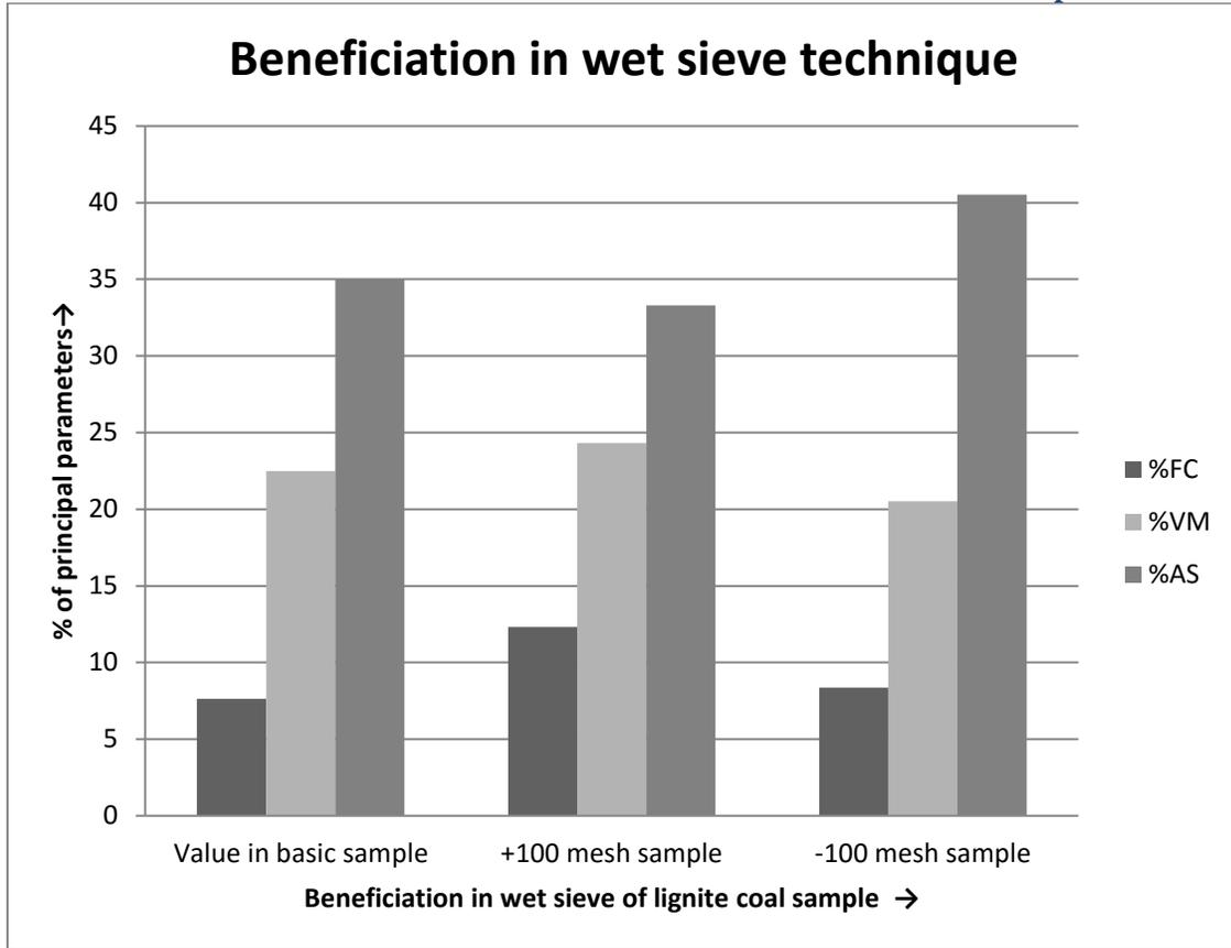
*Fig. 3 The representation of beneficiation in wet sieve Technique for +100 mesh size and -100 meshes rang in 0.298mm to 55 mm.*
