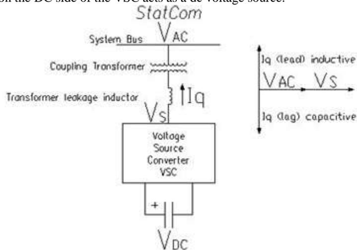
Fig.1 Schematic Configuration of STATCOM
