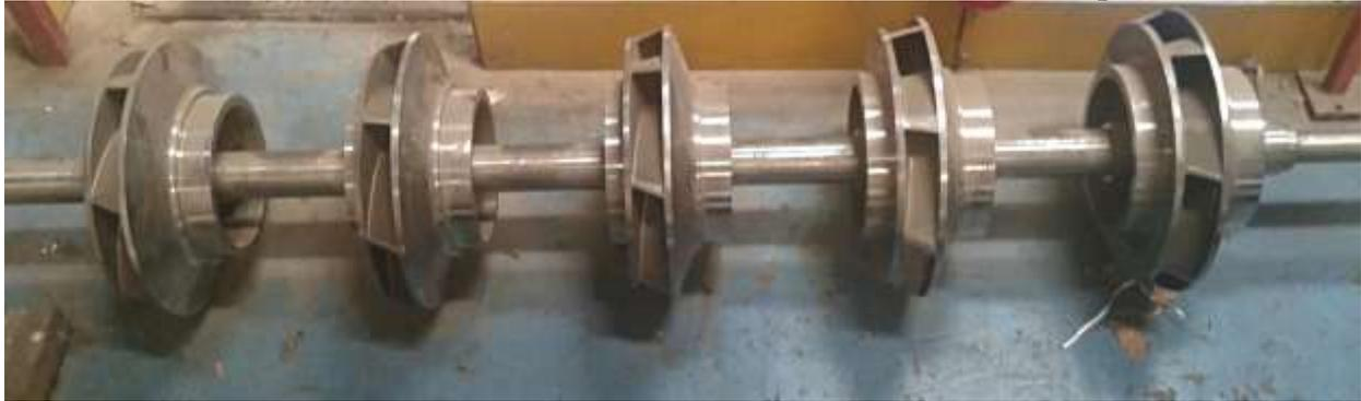
*Fig 8.Boiler feed pump rotor*
