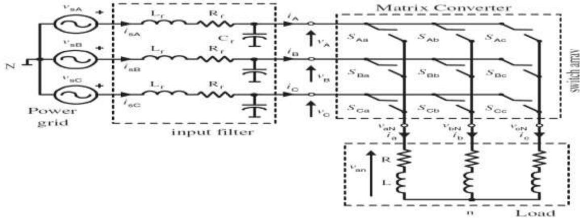
Fig2.2: Matrix Converter circuit
