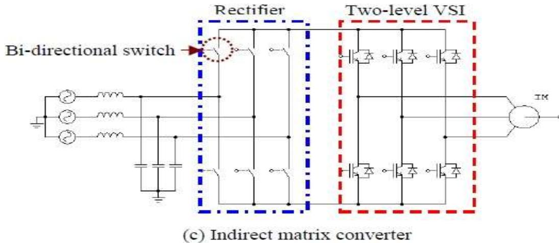
Fig2.1: (a) Direct matrix converter (b) Bi-directional Switches (c) indirect matrix converter
