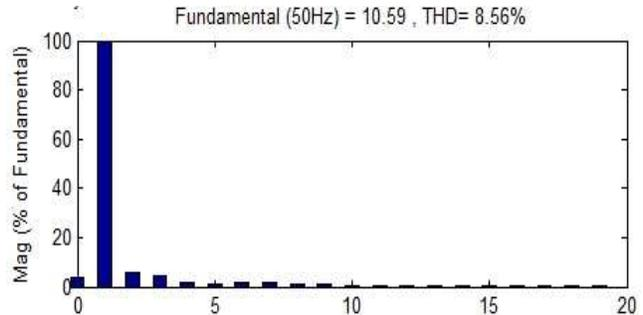
Fig 5.2 : Harmonic spectrum analysis of linear load current (PI controller)
