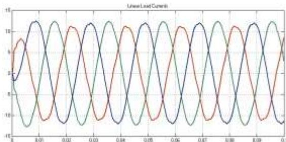
Fig. 5.3: Linear load current (Fuzzy Logic Controller)
