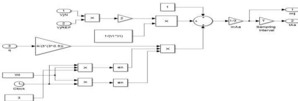
Fig 2.3: Simulink model of matrix converter to generate duty cycle for one output phase
