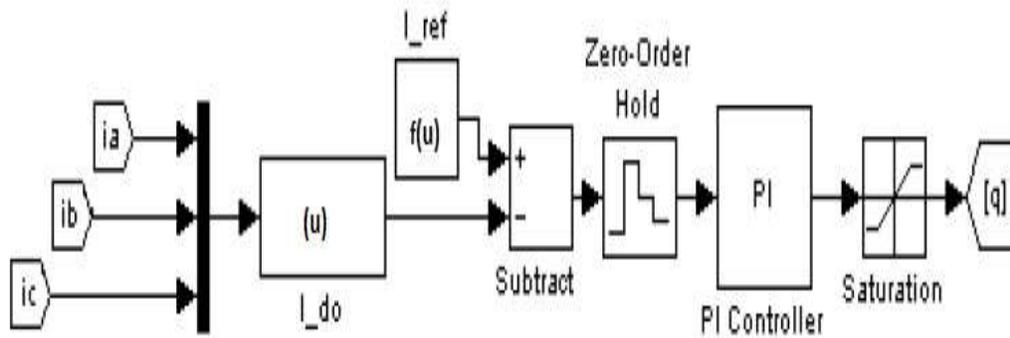
Fig 4.2: Simulink diagram of PI controller based feedback system
