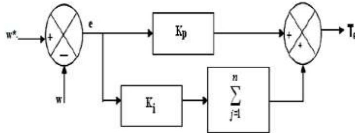
Fig 3.1: Block diagram of PI controller
