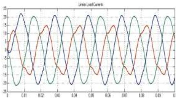
Fig.5.7: Linear load current (Fuzzy Logic Controller)
