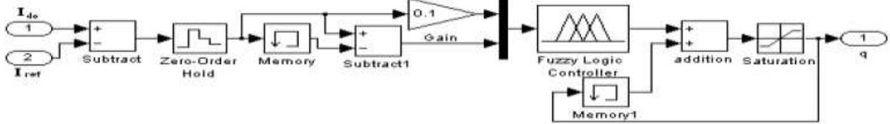
Fig 4.3: Simulink diagram of FLC based feedback system
