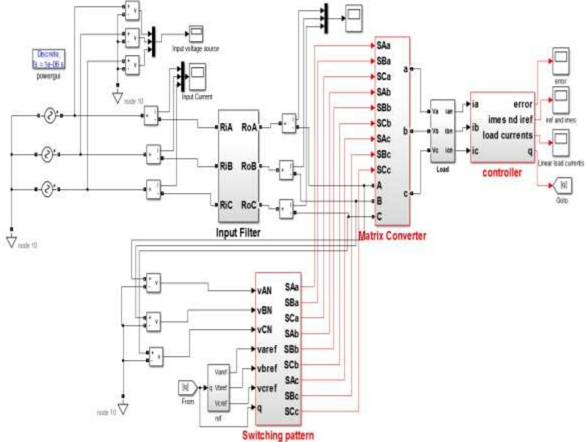
Fig 4.1: Simulink Model Of Controllers Fed To Matrix Converter
