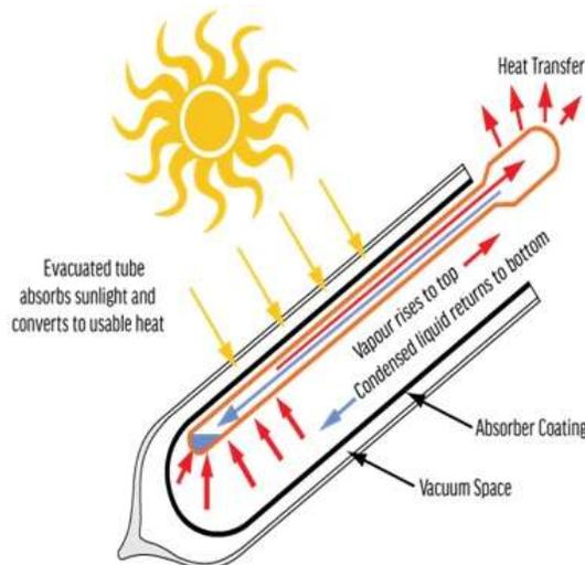
Schematic representation of evacuated tube collector collecting solar radiation [3]
