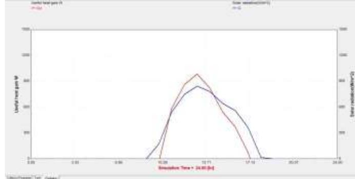
*Variation of solar radiation and useful heat gain with respect to time*
