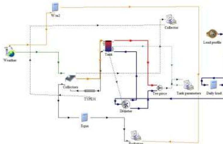
**TRNSYS model diagram for solar water heating with water as HTF**
