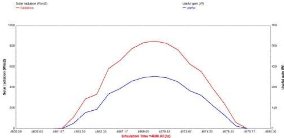
*Solar radiation and Useful energy gain of solar greenhouse*
