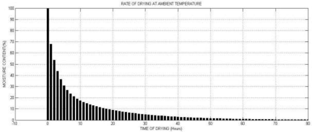
*Rate of drying of rice at ambient temperature*
