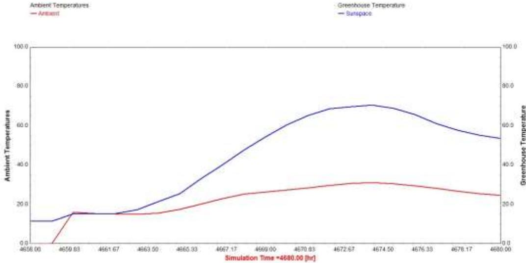
*Ambient temperature and outlet temperature solar greenhouse*
