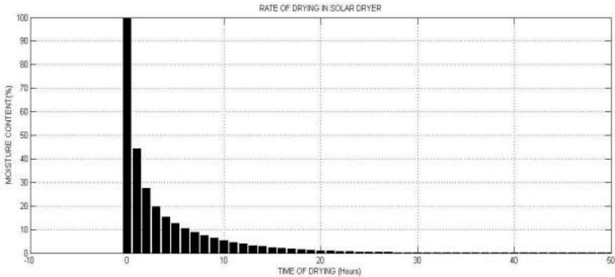
*Rate of drying of rice in solar dryer*
