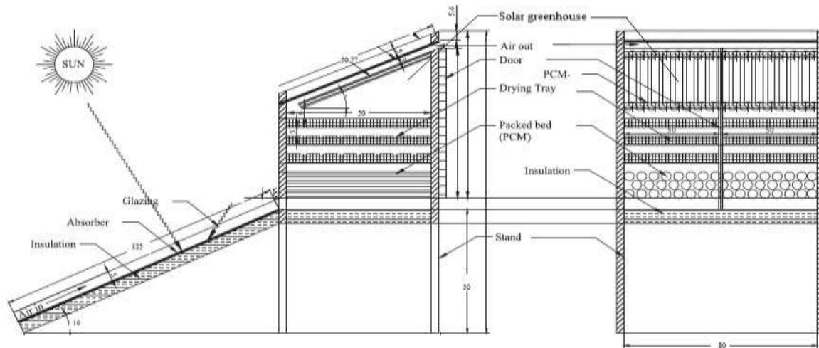
*Mixed mode solar dryer with PCM storage [6]*
