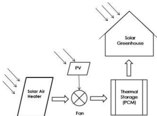
*Block diagram of mixed mode solar dryer*
