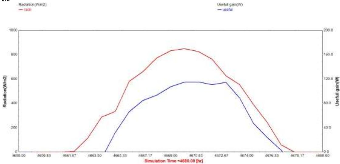
*Solar radiation and Useful heat gain of solar air heater*
