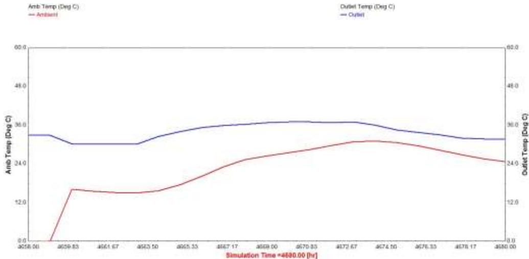
*Ambient temperature and outlet temperature of solar air heater*
