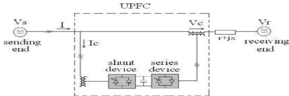
Figure 2: A Basic UPFC functional scheme
