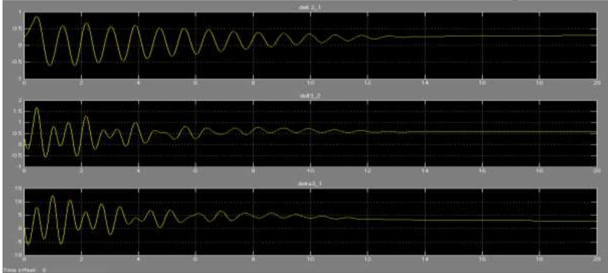
Figure shows the relative angular positions for delt2\_1, delt3\_2and delt3\_1 for multi-machine system with STATCOM controller placed between Bus 8 and Bus 9 and fault taking place between Bus 5 and Bus 7.The total simulation time taken is 20 sec.
