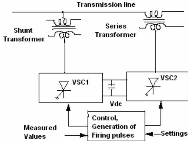
Figure 1: Block Diagram of UPFC
