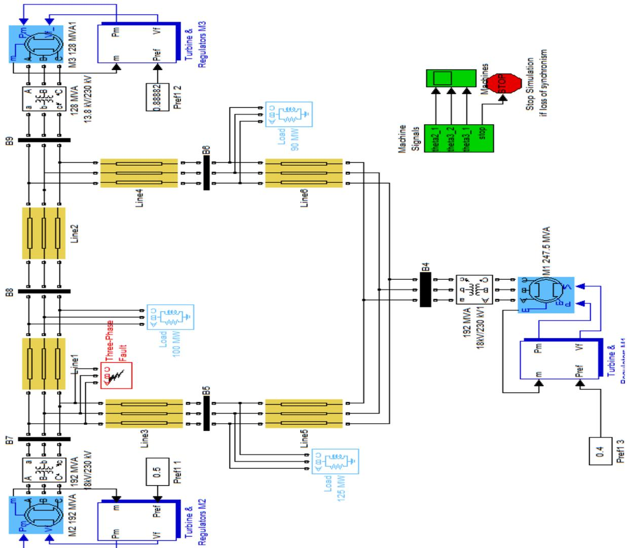
a) STATCOM is placed between Bus 8 and Bus 9
