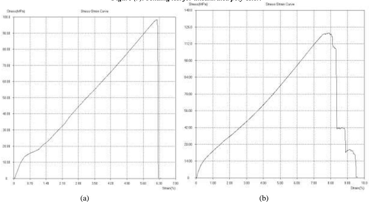
Figure (10): bending test curve for unsaturated poly-ester reinforced with (a) chopped fiberglass (b) 0/90 fiberglass.
