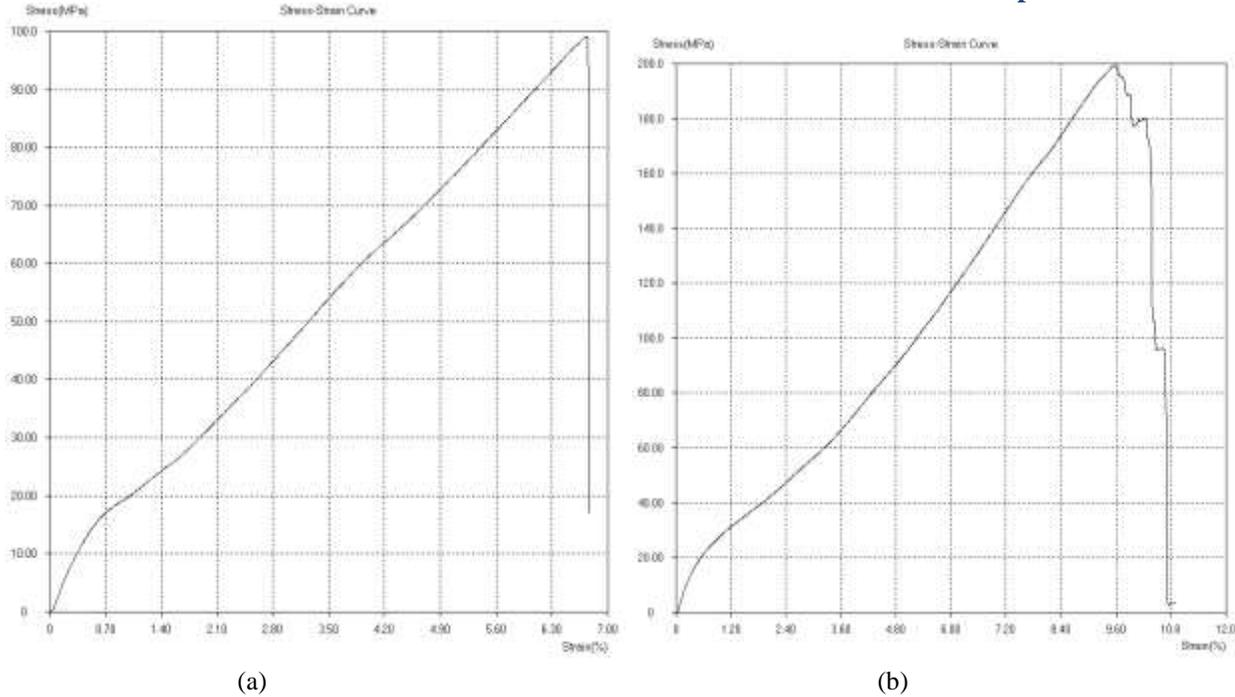
Figure (11): bending test curve for unsaturated poly-ester reinforced with (a) chopped fiberglass (b) 0/90 fiberglass and 3wt% of nanoclay.
