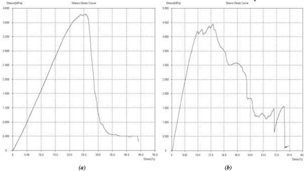
Figure (7): tensile test curve for unsaturated poly-ester reinforced with (a) chopped fiberglass (b) 0/90 fiberglass and 3% of nanoclay.
