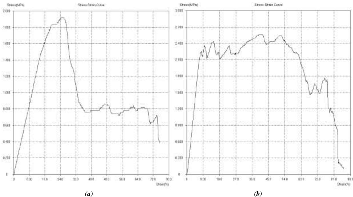
Figure (6): tensile test curve for unsaturated poly-ester reinforced with (a) chopped fiberglass (b) 0/90 fiberglass.
