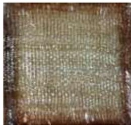
*Figure (3): UPE reinforced with 0/90 fiberglass*
