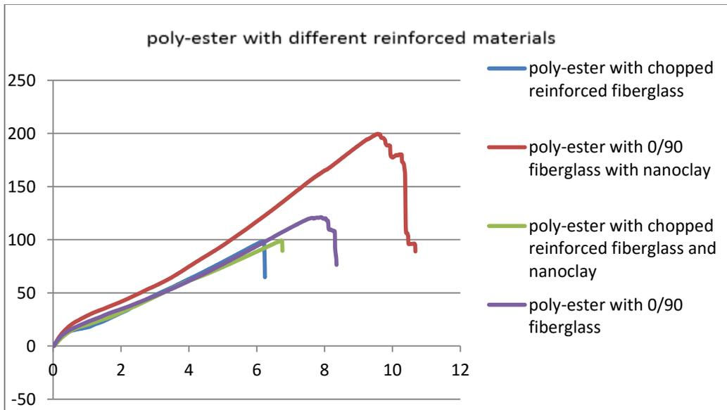
Figure (12): bending test results
