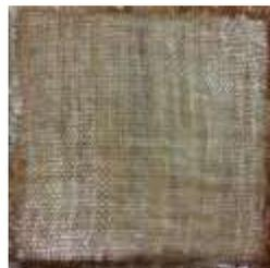
*Figure (5): UPE reinforced with 0/90 fiberglass and nanoclay*
