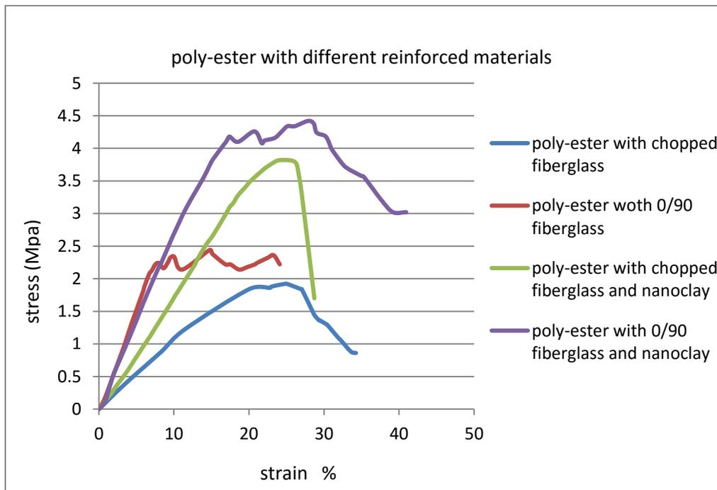
Figure (8): tensile test results
