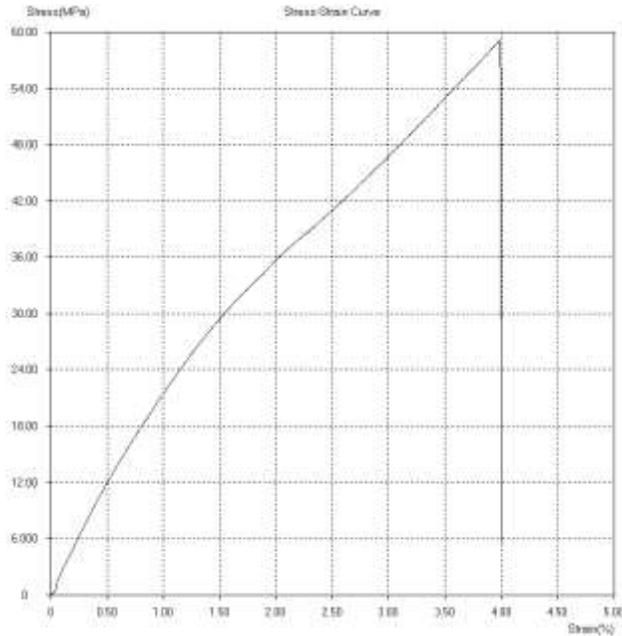
Figure (9): bending test for unsaturated poly-ester.
