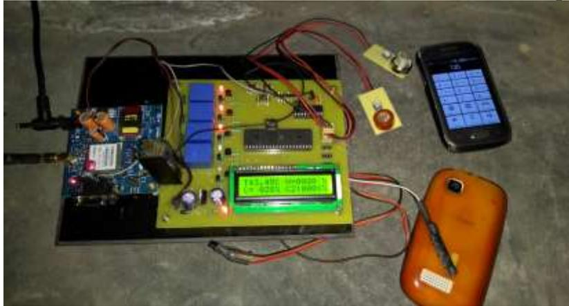
*Fig. 5.5 three street lights are ON (for S3: dial 3)*
