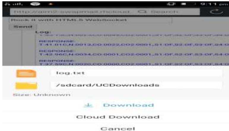
*STEP7: Downloaded file shows variation in result of atmospheric parameters such as temperature- T, CO- C, CO2- C2, Noise- N and controlling street light ON/OFF delay duration of 3 sec (S1 and S2 gets ON for few sec)*
