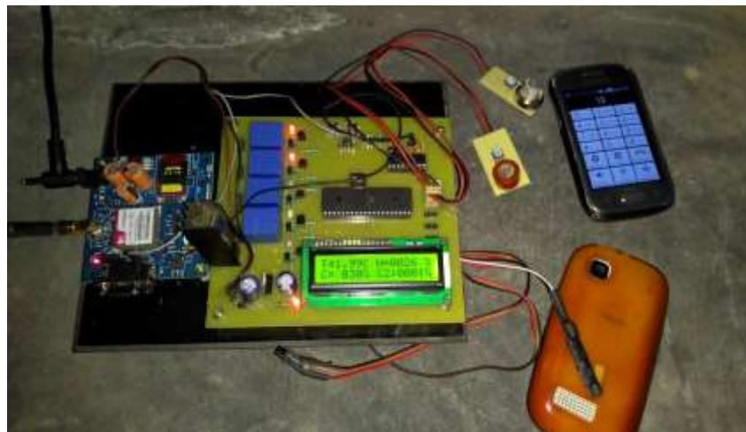
*Fig. 5.4 street light 1<sup>st</sup> and 2<sup>nd</sup> both ON (for S2: dial 3)*
