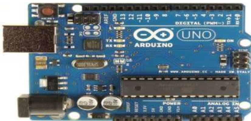
*Figure 6.1 Arduino UNO R3 Board*
