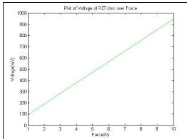
**Figure 5.Voltage versus Static force**
