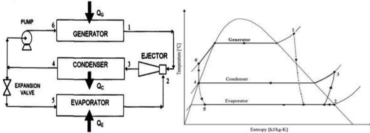
As we know that the domestic vapour absorption refrigeration systems works between 0.5 to 1.0 kg/min of refrigerant flow rate (from design point of view) .Hence, taking mass flow rate of refrigerant (R-11) in power loop is 0.65 kg/min. (refer previous figure)
