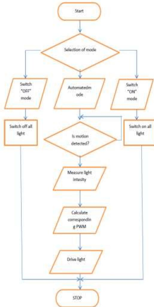
**Fig 3: Flowchart of Intelligent Lighting control algorithm**
