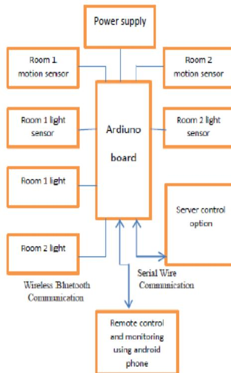
**Fig 4: Block diagram of Intelligent Lighting System**
